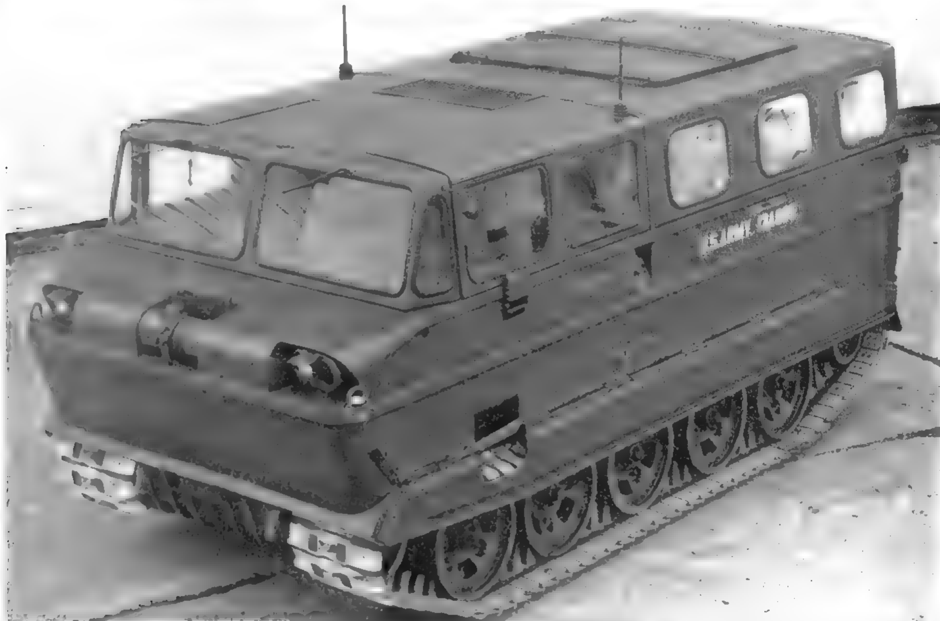
Though not actually an M116, but an T116E1 pilot vehicle, this vehicle shows how the the optional rear hardtop enclosure was fitted to the vehicle. The hatch in the roof allowed the overhead loading of cargo. (U.S. Army photo)
